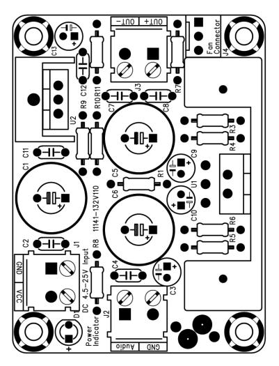
J1 is for power input. J2 is for audio input. J3 is for audio output. What you need to do is to solder terminal blocks.
